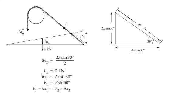
$$P \sin 30^{\circ} \times \Delta x \sin 30^{\circ} = 2 \times \frac{\Delta x \sin 30^{\circ}}{2}$$
