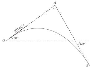
Let, *t* is the time from the instant of projection, when the particle will move perpendicular to its initial direction.
