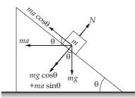
For maximum acceleration, the applied force should be such that it balances the effect of frictional force and gravity. Hence applied force,
