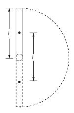
Linear speed of the free end at given instant,  $v = l\omega$
