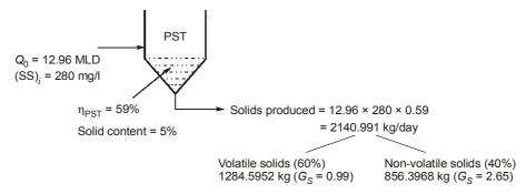
5 kg of solids  $\simeq$  100 kg of sludge 5 kg of solids  $\cong$  95 kg of water 1 kg of solids  $\cong$  19 kg of water
