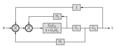
Now  $\frac{G_1G_2}{1+G_1H_1}$  forms a positive feedback loop with  $H_2$  and that loop is in cascade with  $G_3$ . The
