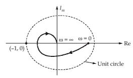
Polar plot does not cross unit circle, for all values of  $\omega$  (0 to  $\infty$ ), magnitude will be less than unity. In this case, gain crossover frequency does not exist and phase margin becomes  $\infty$ .
