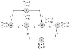
Total float =  $T_L$  for head event –  $T_E$  for tail event – duration of activity Total float of AB = 8 - 0 - 5 = 3 weeks Total float of CE = 11 - 6 - 3 = 2 weeks Free float =  $T_E$  for head event –  $T_E$  for tail event – Duration of activity Free float of EF = 18 - 9 - 7 = 2 weeks :. Total float AB + Total float of CE + Free float of EF = 3 + 2 + 2 = 7 weeks
