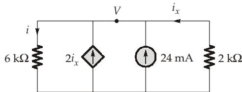
$$\text{Applying KCL, } i = 2i_x + 24 \text{ mA} + i_x \dots (\text{i})$$
