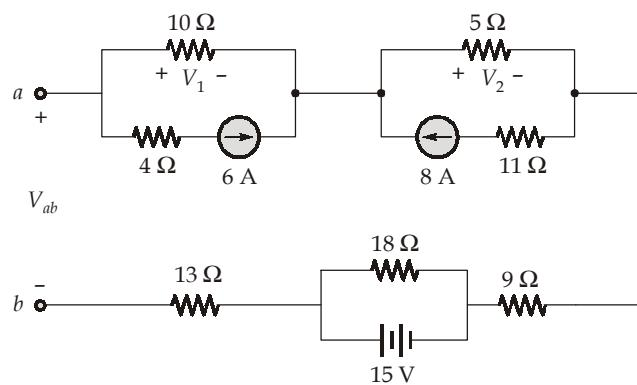
$$V_{ab} = V_1 + V_2 - 15 \text{ V}$$
