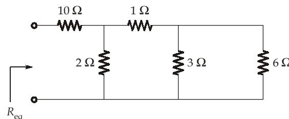
$$\therefore R_{eq} = 10 \Omega + 2 \Omega \parallel (1 + 3 \Omega \parallel 6 \Omega)$$
