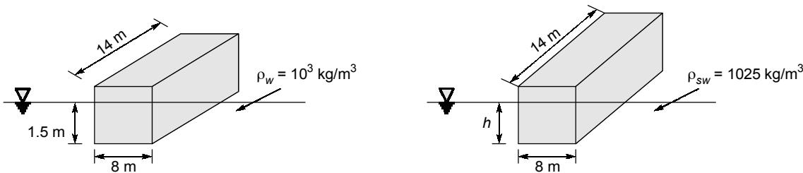
In both the cases the weight of rectangular portion remains same and balanced by Buoyancy force. So,
