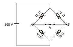
It is easy to calculate  $I_L$  by calculating Thevening equivalent across the terminals A and B. To determine  $V_{Th}$ :
