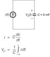
For 0 < t < 5; Unit step current is applied; voltage will increase linearly. For 5 < t < 10; No current is applied, hence open circuit, the capacitor will hold the charge. For 10 < t < 15; again capacitor's voltage increases linearly. From above analysis,
