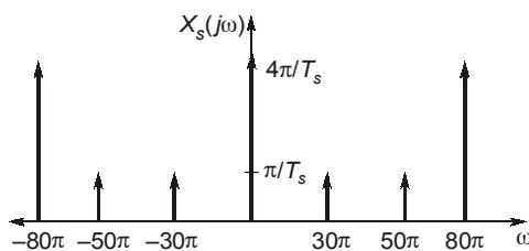
$$X_s(j\omega) = 40 \sum_{m=-\infty}^{\infty} [4\pi\delta(\omega - 80\pi) + \pi\delta(\omega - 50\pi - 80\pi m) - \pi\delta(\omega + 50\pi - 80\pi m)]$$
