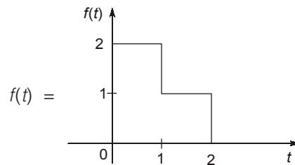
The signal  $f(2t - 3)$  involves time scaling and time shifting.
