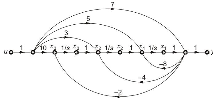
$$\begin{aligned}\dot{x}_3 &= 10u - 2x_1 \\ \dot{x}_2 &= 3u + x_3 - 4x_1 \\ \dot{x}_1 &= 5u - 8x_1 + x_2 \\ y &= 7u + x_1\end{aligned}$$
