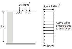
$$k_a = \frac{1-\sin\phi}{1+\sin\phi} = \frac{1-\sin 28^\circ}{1+\sin 28^\circ} = 0.36$$
