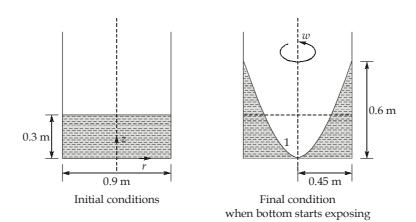
Apply forced vortex motion equation at points (1) and (2)
