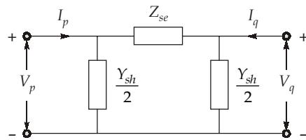
$$Y_{\text{bus}} = \begin{bmatrix} \frac{1}{Z_{se}} + \frac{Y_{sh}}{2} & -\frac{1}{Z_{se}} \\ -\frac{1}{Z_{se}} & \frac{1}{Z_{se}} + \frac{Y_{sh}}{2} \end{bmatrix}$$
