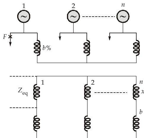
Equivalent impedance  $Z_{eq}$  between the zero potential bus and the fault point is
