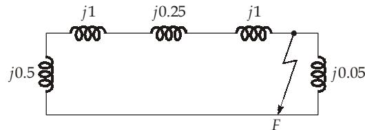
$$\begin{aligned} Z_1 &= Z_2 \\ &= j 2.75 \parallel j 0.5 = j 0.423 \text{ p.u.} \end{aligned}$$
