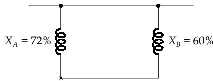
$$I_{\text{base}} = \frac{\text{MVA}}{\sqrt{3} \text{ kV}} = \frac{45 \times 10^6}{\sqrt{3} \times 15 \times 10^3} = 1732.05 \text{ A}$$
