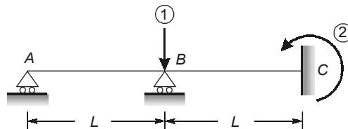
The elements of the flexibility matrix are obtained by applying unit values of redundants at the coordinates one after the other as shown below.
