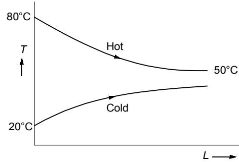
$$\text{LMTD} = \frac{\Delta T_1 - \Delta T_2}{\ln\left(\frac{\Delta T_1}{\Delta T_2}\right)} = \frac{60 - 14.325}{\ln\left(\frac{60}{14.325}\right)} \approx 32^\circ\text{C}$$
