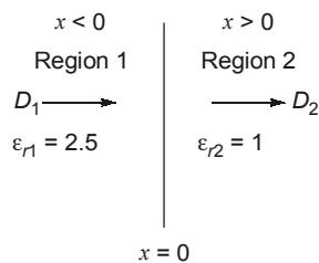
1. Normal component of electric field density for source free region is continuous,
