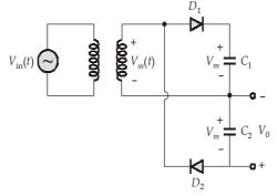
The circuit represents a voltage doubler circuit, if the voltage was taken by adding voltages of both the capacitors, but to calculate  $V_0$  we have to find the voltage stored on a single capacitor. Thus, comparing from the above figure,
