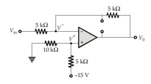
$$V_0 = -\frac{5}{5} \times V_{\text{in}} = -V_{\text{in}} \text{ (for } V_{\text{in}} < -10 \text{ V)}$$
