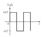
For negative cycle  $V_{\rm in}$  < 3.2 V always, thus the MOSFET  $M_1$  will be OFF and diode  $D_1$  will be ON
