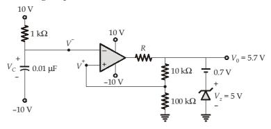
$$V^{+} = V_{0} \times \frac{100 \text{ k}\Omega}{(10+100) \text{ k}\Omega}$$
