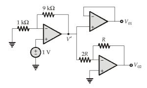
$$V' = \left(1 + \frac{9 \,\mathrm{k}\Omega}{1 \,\mathrm{k}\Omega}\right) \times 1 \,\mathrm{V} \qquad (\because \text{ non-inverting amplifier})$$
