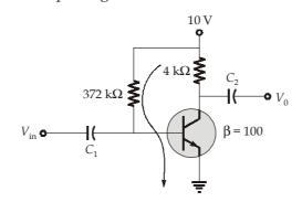
$$I_B = \frac{10 - 0.7}{372 \text{ k}\Omega} = 25 \,\mu\text{A}$$
