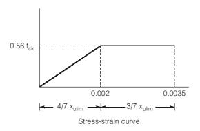
According to IS - 456, the partial safety of factor for stress in concrete is 1.5 and maximum stress according to this factor is 0.45  $f_{ck}$  but for new assigned factor (= 1.2) this value changes to 0.558  $f_{ck}$
