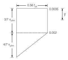
To calculate limiting moment, we need to calculate the lever arm Centroid of compressive force,
