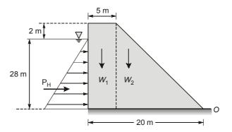
$\gamma_c = 24 \text{ kN/m}^3$  (Considering inside length of dam as unity)
