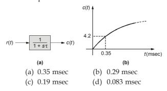
**Q.19** A unity negative feedback control system has the closed loop transfer function,
