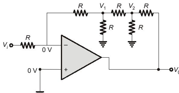
$$\frac{3V_1}{R} = \frac{V_2}{R}$$
