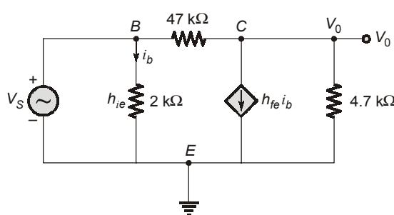
$$i_b = \frac{V_s}{h_{ie}} = \frac{V_s}{2\text{k}\Omega}$$
