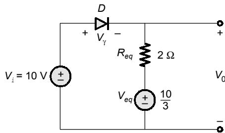
$$V_{eq} = \frac{-\frac{10}{6} + \frac{10}{3}}{\frac{1}{6} + \frac{1}{3}} = \frac{10 \times \frac{3}{18}}{\frac{9}{18}} = \frac{10 \times 3}{9} = \frac{10}{3} \text{ volts.}$$
