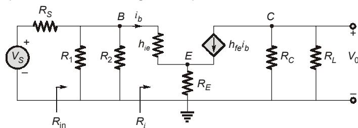
$$V_0 = -h_{fe} i_b (R_C \parallel R_L) = -h_{fe} i_b R'_L$$
