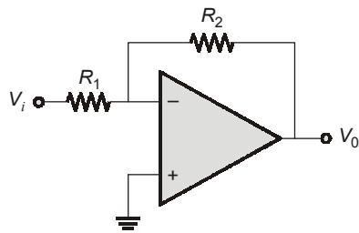
$$V_0 = -V_i \left( \frac{R_2}{R_1} \right)$$
