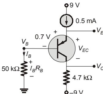
$$I_C = \frac{\beta}{\beta + 1} (I_E) = \frac{49(0.5)}{50} \text{ mA} = 0.49 \text{ mA}$$
