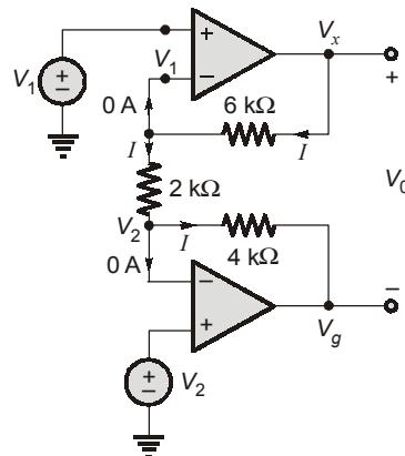
$$V_0 = I(6 \text{ k} + 2 \text{ k} + 4 \text{ k}) = I(12 \text{ k})$$
