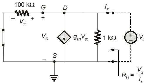
$$I_x = g_m V_\pi + \frac{V_\pi}{100 \text{ k}\Omega} + \frac{V_\pi}{1 \text{ k}\Omega}$$
