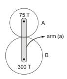
As gear B is fixed here,  $N_B = 0$ ,  $y - x \left(\frac{75}{300}\right) = 0$
