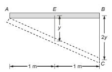
Now using the principle of virtual work done, if C.G. of beam *AB* shifts by an amount 'y' then end *B* must shift by '2y' (using similar triangles).
