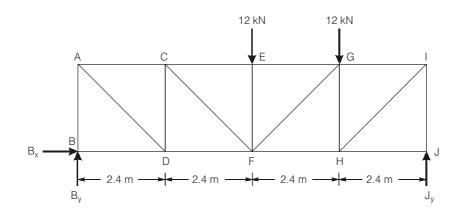
$$\begin{split} \Sigma M_{J} &= 0, \\ 12 \times 4.8 + 12 \times 2.4 &= B_{y} \times 9.6 \\ B_{y} &= 9 \text{ kN} \\ \Sigma F_{y} &= 0, \\ B_{y} + J_{y} &= 24 \text{ kN}, \quad J_{y} = 15 \text{ kN} \\ F_{CD} + 9 &= 0 \\ F_{CD} &= -9 \text{ kN} \\ \Sigma M_{C} &= 0, \\ -9 \times 2.4 + F_{DF} \times 1.8 &= 0 \end{split}$$
