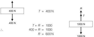
This is the reaction from the ground and it is the same force with which the 1000 N block press against the floor.
