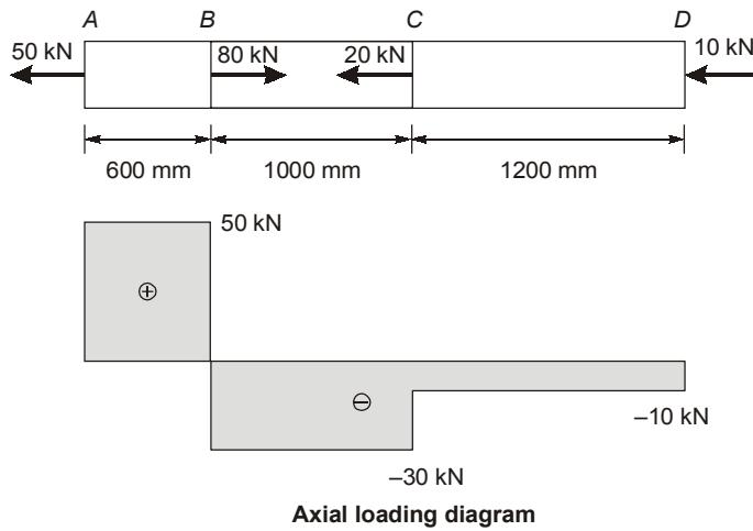
**Part AB:** The section of the bar in this part is subjected to a tension of 50 kN.
