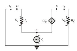
$$V_0 = -\beta i_b R_c$$
