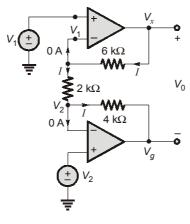
$$V_0 = I(6 \text{ k} + 2 \text{ k} + 4 \text{ k}) = I(12 \text{ k})$$
