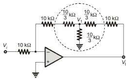
Applying KCL at inverting node
