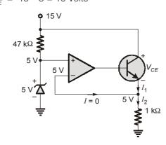
Power dissipated in transistor
