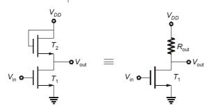
Calculating  $R_{\text{out}}$  of  $T_2$
