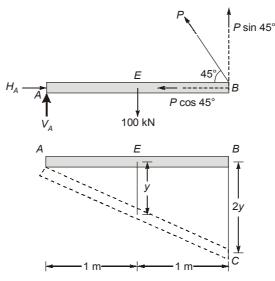
Now using the principle of virtual work done, if C.G. of beam AB shifts by an amount 'y' then end B must shift by '2y' (using similar triangles).
