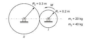
Moment of inertia,  $I_2 = \frac{m_1 R_1^2}{2} = \frac{20 \times 0.2^2}{2} = 0.4 \text{ kgm}^2$
