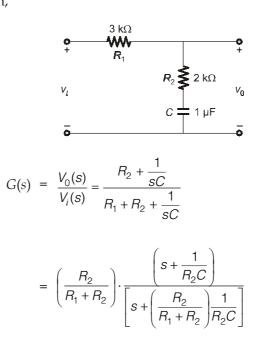
$$\alpha = \frac{R_1 + R_2}{R_2} = \frac{3 \,\mathrm{k}\Omega + 2 \,\mathrm{k}\Omega}{2 \,\mathrm{k}\Omega} = \frac{5}{2} = 2.50$$
