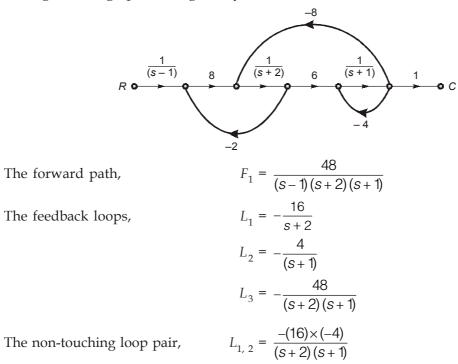
:. The closed loop transfer function using Mason's gain formula is,
