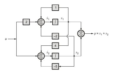
As per the block diagram, state equations are,
