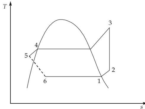
Degree of superheat at suction  $t_2 - t_1 = 15 - (-15) = 30\text{K}$
