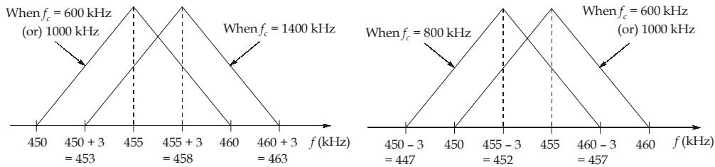
So, the minimum bandwidth required by the IF amplifier can be given by,
