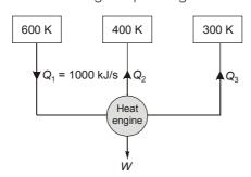
$$\begin{array}{c} Q_1 = Q_2 + Q_3 + W \\ 1000 = Q_2 + Q_3 + 50 \\ \\ \Rightarrow Q_2 + Q_3 = 950 \text{ kJ/s} \\ \\ \hline \sum \frac{Q}{T} = 0 \end{array} \qquad \text{[Claussius inequality] [for reversible process]}$$
