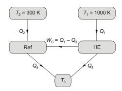
$$\Rightarrow W_c = Q_2 \left( \frac{T_3 - T_2}{T_2} \right) \qquad \dots (ii)$$
