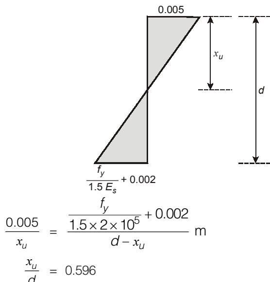
Limiting depth of neutral axis using Fe 415 according to IS 456:2000 = 0.48 d
