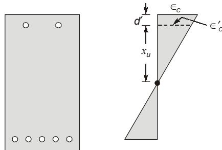
Maximum strain in concrete = 0.0035
