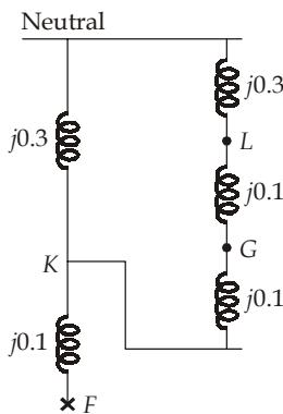
Total per unit impedance from generator neutral upto fault point F
