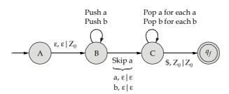
$$L = \left\{ \underbrace{w}_{\text{push}} \underbrace{x}_{\text{skip}} \underbrace{w^{R}}_{\text{pop}} \middle| w \in (a+b)^{*} x \in (a+b) \right\}$$
