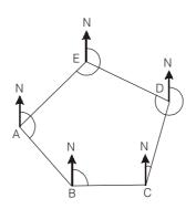
Correct FB of DE =  $134^{\circ} 45' + 180^{\circ} = 314^{\circ} 45'$
