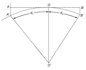
Let A and B be the two triangulation stations and let O be the point of tangency on the horizon. Let  $A'A = C_1 = 9000 \text{ m} = 9 \text{ km}$
