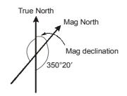
Since the magnetic bearing of the Sun is 350° 20′, it is at the North of the place and hence the true bearing of the Sun, which is on the meridian, will be 360°.
