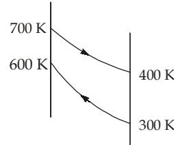
Counter flow is chosen because cold fluid exit temperature (600 K) is greater than hot fluid exit temperature (400 K)
