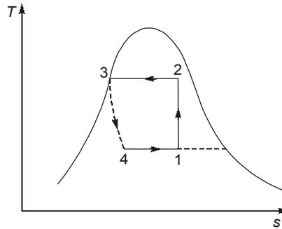
$$s_1 = s_{f_1} + \frac{x_1 h_{fg1}}{T_1} = 0.5443 + \frac{x_1 \times 1297.68}{263} = 0.5443 + 4.934 x_1$$
