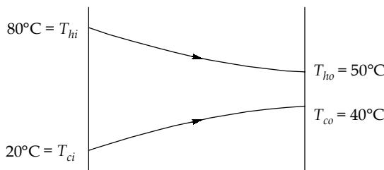
$$\Delta T_1 = 80^\circ\text{C} - 20^\circ\text{C} = 60^\circ\text{C}$$
