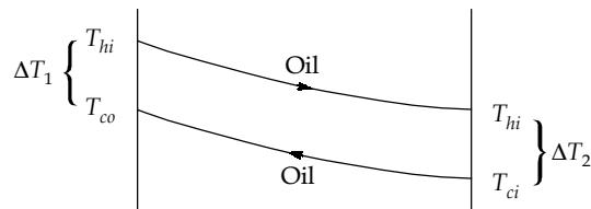
$$\Delta T_1 = 70^\circ\text{C} - 40^\circ\text{C} = 30^\circ\text{C}$$
