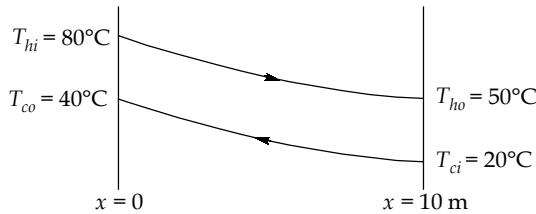
$$\Delta T_1 = 80^\circ\text{C} - 40^\circ\text{C} = 40^\circ\text{C}$$
