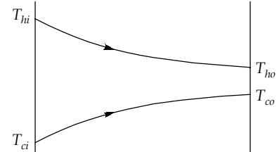
$$\text{(LMTD)}_{\text{parallel}} = \frac{\Delta T_1 - \Delta T_2}{\ln\left(\frac{\Delta T_1}{\Delta T_2}\right)} = \frac{50^\circ\text{C} - 5^\circ\text{C}}{\ln\left(\frac{50}{5}\right)}$$
