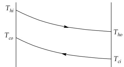
$$(\text{LMTD})_{\text{counter}} = 26.804^\circ\text{C}$$
