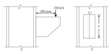
Direct shear stress,  $q = \frac{P}{2t \times d}$
