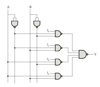
$$Y = \overline{S}_{1}\overline{S}_{0}(I_{0}) + \overline{S}_{1}S_{0}(I_{1}) + S_{1}\overline{S}_{0}(I_{2}) + S_{1}S_{0}(I_{3})$$
