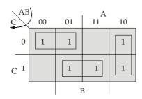
$$F(A, B, C) = \overline{A}\overline{C} + BC + \overline{A}B$$
