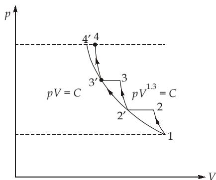
$$\begin{aligned}\text{Compressor work, } W_{\text{poly}} &= N \left( \frac{n}{n-1} \right) R T_1 \left[ \left( \frac{p_4}{p_1} \right)^{(n-1)/nN} - 1 \right] \\ &= 3 \left( \frac{1.3}{1.3-1} \right) \times 0.287 \times 298 \left[ \left( \frac{3000}{96} \right)^{(1.3-1)/1.3 \times 3} - 1 \right]\end{aligned}$$
