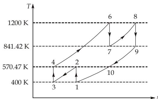
For ideal conditions, work output of each turbine and work input of each compressor would be same.
