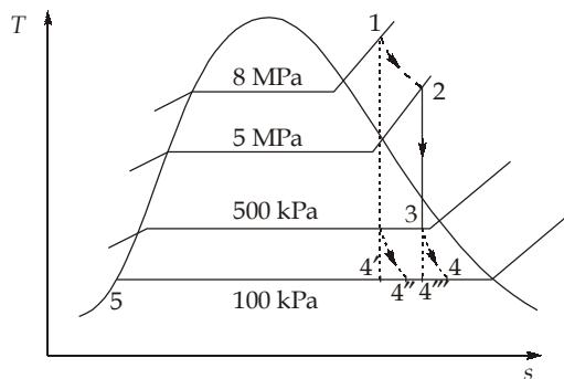
On removal of valve, steam at state 1 will expand directly to 4' hence the quality of steam at exit will decreases,
