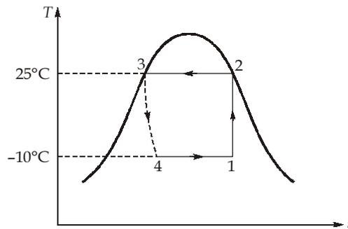
$$\begin{aligned} s_2 &= (s_g)_{25^\circ\text{C}} = 5.0391 \text{ kJ/kgK} \\ s_2 &= s_1 = (s_g)_{-10^\circ\text{C}} + x(s_{fg})_{-10^\circ\text{C}} \\ 5.0391 &= 0.5443 + x(5.4770 - 0.5443) \\ x &= 0.9112 \end{aligned}$$
