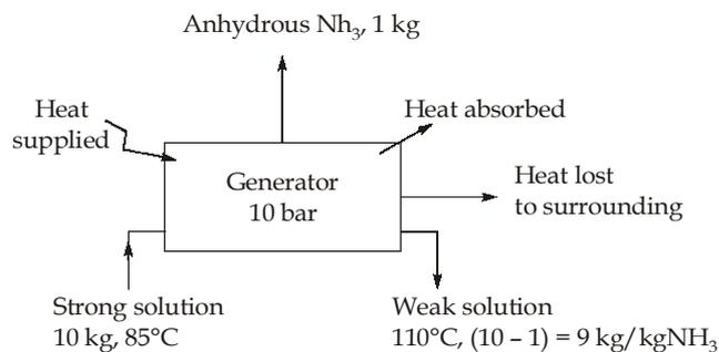
**Energy balance:** Heat of strong ammonia-aqua + Heat from heating source = Heat of anhydrous  $NH_3$  vapour + Heat of weak solution + heat absorbed + heat lost to surrounding.
