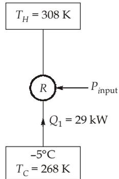
$$\text{Actual COP} = \frac{1}{3} \times \text{ideal COP} = \frac{1}{3} \times \left( \frac{T_C}{T_H - T_C} \right) = \frac{1}{3} \left( \frac{268}{308 - 268} \right)$$
