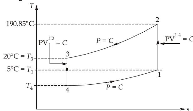
$$\begin{aligned} W_{\text{compressor}} &= C_p(T_2 - T_1) \\ &= 1.005 (463.85 - 278) \\ &= 186.78 \text{ kJ/kg} \end{aligned}$$
