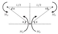
$$\begin{aligned} W_i &= W_E \\ \Rightarrow & 4M_p\theta &= w_u \left(\frac{1}{2} \times L \times \frac{L}{2}\theta\right) \\ \Rightarrow & w_u &= \frac{16M_P}{L^2} \end{aligned}$$
