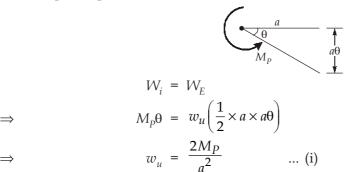
For collapse of part AB, plastic hinges will be developed at A, B and at mid point of AB.
