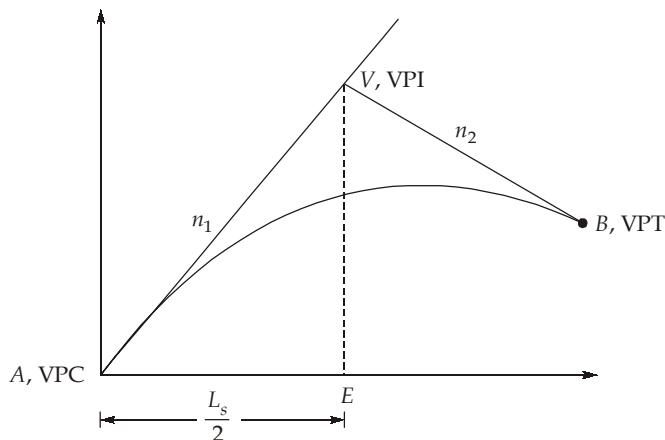
$$\begin{aligned} RL_A &= RL_V - \frac{L_s}{2} \times n \\ &= 75 - \frac{474.73}{2} \times 0.015 = 71.44 \text{ m} \end{aligned}$$
