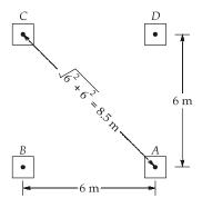
For footing A, B, C, D, the  $\frac{r}{Z}$  ratios are 0,  $\frac{6}{3}$ ,  $\frac{6}{3}$  and  $\frac{8.5}{3}$  respectively.
