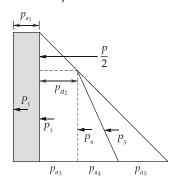
$$p_{a_1} = K_a \times q = \frac{1}{3} \times 14 = 4.67 \text{ kN/m}^2$$
