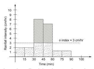
Hatched portion shows the total runoff and dotted portion shows the total infiltration.
