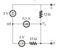
$V_{\rm Th}$  is the voltage dropped by 12  $\Omega$  resistor  $V_{\rm Th} = V_a - V_b = 2 - V_b$
