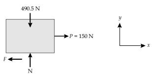
Because F < Fmax, we conclude that the block is in static equilibrium and correct value of friction force,
