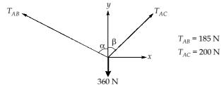
$$T_{AB} \sin \alpha = T_{AC} \sin \beta$$
