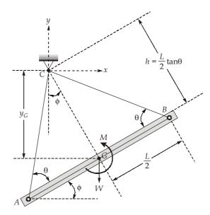
Considering the fixed point C as origin of rectangular coordinate system. Point *G*:
