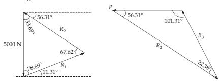
Applying Lami's theorem for block A
