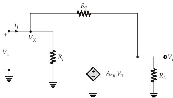
$$R_{in} = \frac{V_1}{i_1}$$
