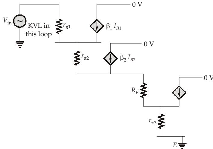
$$V_{in} = I_{B1} r_{\pi 1} + r_{\pi 2}(1 + \beta_1)I_{B1} + R_E(1 + \beta_2)I_{B2} + r_{\pi 3}(1 + \beta_2)\beta_1 I_{B1}$$
