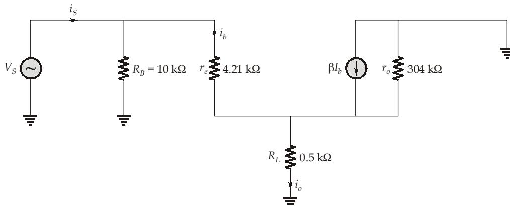
$$i_o = \frac{r_o}{r_o + R_L} (\beta + 1) i_b$$
