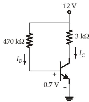
$$I_B = \frac{12 - 0.7}{470 \text{ k}} = 24.04 \mu\text{A}$$
