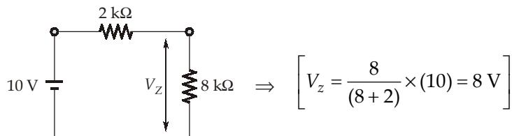
At Breakdown,  $I_z = I_{z \min}$  ( $V_s = 10 \text{ V}$ )
