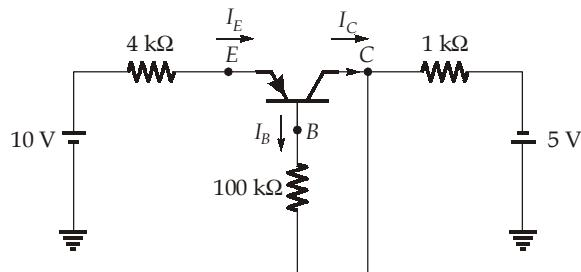
$$I_E = \frac{10 - V_E}{4 \text{ k}\Omega} = \frac{10 - 4}{4 \text{ k}\Omega} = 1.5 \text{ mA}$$
