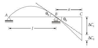
Now  $\Delta C_1$  is produced due to deflection of C as caused due to deformation of AB,
