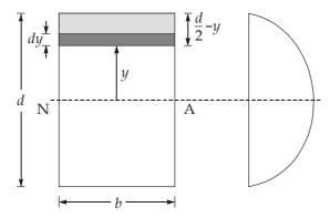
Shear stress at 'y' distance from neutral axis.
