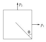
The maximum shear stress will occur at 45° plane from principle plane
